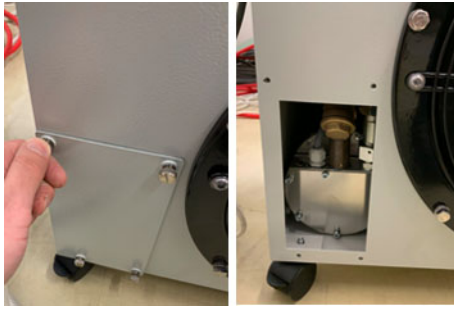
[1]: Cover to access filter strainer
